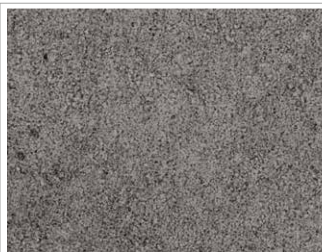
Figure 2B. Regular and fine texture. The homogeneity and uniformity help to extend the shelf life of the dispersed system. (Leica DM 1000- 20x).
